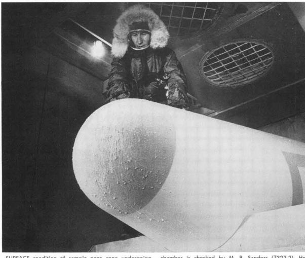
SURFACE condition of sample nose cone undergoing extreme low-temperature test in environmental test
